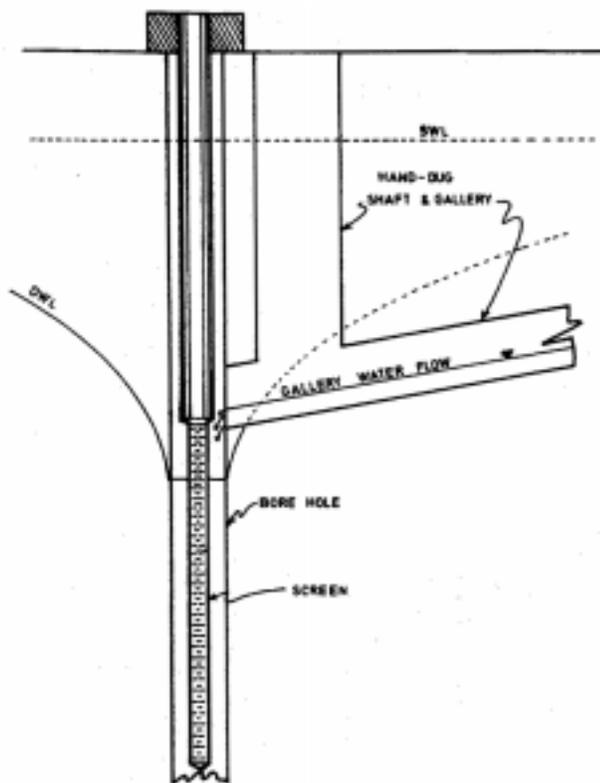
Figure 4. Schematic of a hybrid well.
