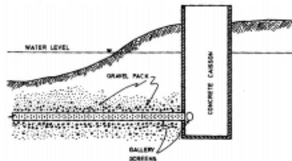
Figure 3. Typical collector well construction.
