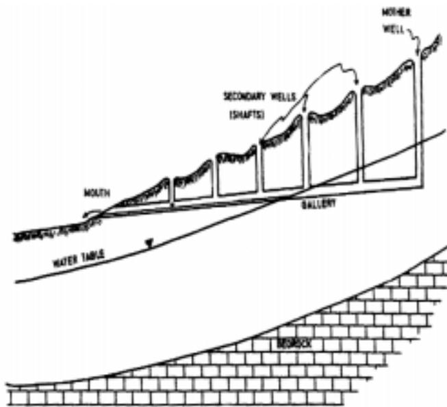
Figure 2. Typical qanat construction.
