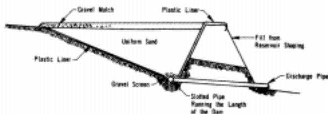
Figure 5. Schematic of an artificial aquifer.
